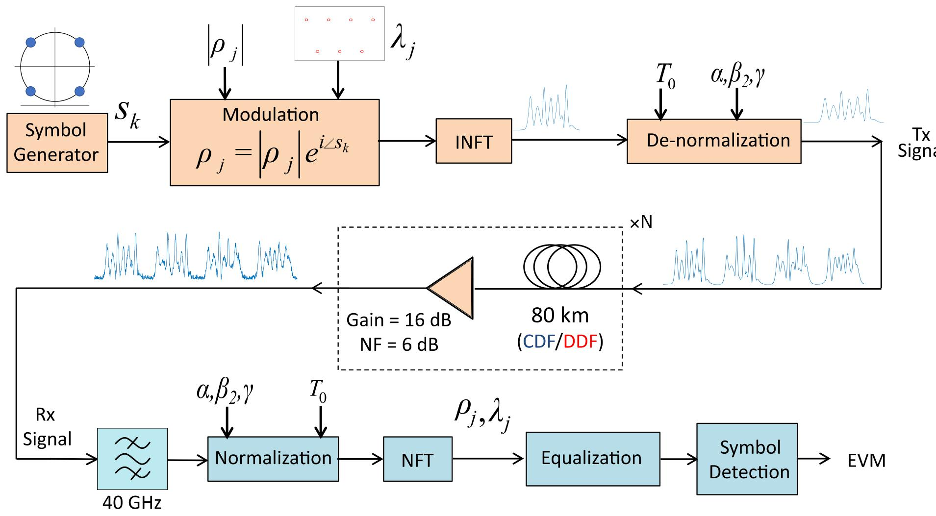
The parameters considered for CDF are average values of corresponding parameters for DDF.
